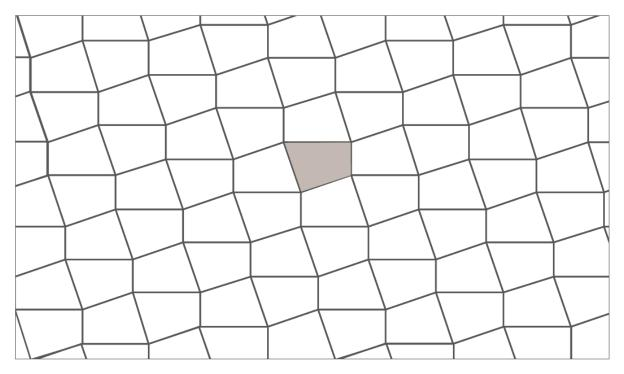
Waste due to elements' perimetric cutting is calculated between 10% and 20% though percentage may slightly vary according to dimension and shape of the surface area to be laid.
