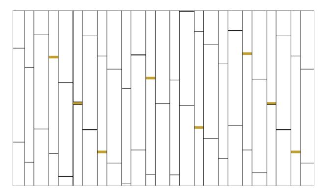
The brass inserts have a width of 90 mm, a length of 20 mm and a thickness of 12,5 mm; they are supplied in the size of 1 piece/m² of hardwood floor.
